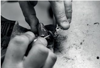
Abrasivne The dust emitted during manual polishing is dangerous for health.
